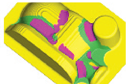
D6R3 re-roughing, ensures D10R5 stock become more regular before semi finishing
